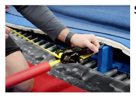
NOTE: If you have trouble ratcheting the Quick Flex Bar, stop and find the end of the strap. Pull the end of the strap with the thick webbing away from the ratchet.
