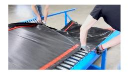
7. Allow the first person to stay 7-10 springs ahead of the second person using the spring tool. The first person should spring all the way to the end of the Tumbl Trak to make sure no D-rings are skipped.
