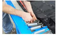
If the bed begins to wrinkle, skip another frame hole where the wrinkle is and continue to spring the bed as before. If you skip a frame hole, make sure to skip the same frame hole on the opposite side to make a smooth, wrinkle-free bed. **Never skip a D-Ring on the Tumbl Trak bed.**
