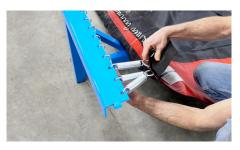
3. Hook the first and second springs into the first D-ring. The third spring should go into the second D-ring and so forth.
