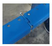
3. Match the knuckles of the rails and insert the bolt to fasten together. Secure with the nut. Make sure the nut is on the inside of the frame. If you purchased a Tumbl Trak in a 5-ft increment, please see further instructions on page 4.
