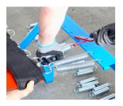
5. Using the spring tool, attach two springs to the first D-ring on the opposite side. Follow the same pattern as the first side, with the third spring going into the second D-ring and so forth.
